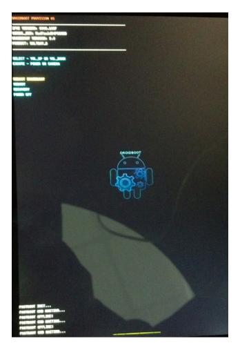
12) Double click file "P802\_flash\_device\_wifi\_only.bat" or "P802\_flash\_device\_lte.bat" in SW image folder. The following CMD window will show up, and begin to flash OS system image.
