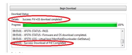
11) After flashing firmware, the tablet device will switch to fastboot mode automatically as the following:
